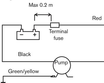
Other electrical devices, eg switch, circuit breaker, must be installed between the pump and the positive (+) lead on the battery (on the red wire).
